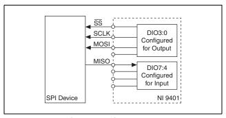
Figure 2. Connecting an SPI Device to the NI 9401
